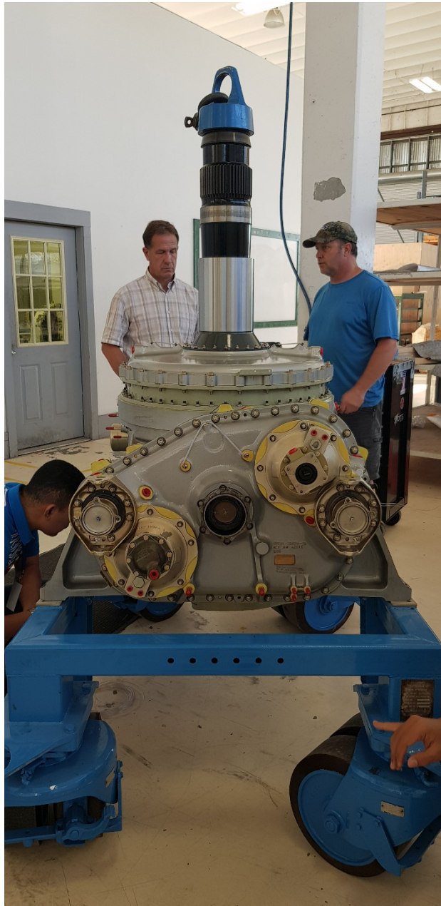
S61A Main Gearbox upgrade from 22000 series to 24000 series in Atlanta
